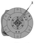
Check the rubber buffers and make sure the holders are secure. The flange holding the buffers (Fig.7.1-1) has to be firmly secured to the unit. If there is a gap seen here, that means the screws securing the holder are loose. The screws have to be tightened immediately to safely operate the machine. Working with loose screws could cause serious damage to the machine. The tightening force of the screws has to be 22-25N.m (16-18ft-lbf).
