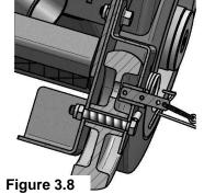
Put the handles of the carriage as shown on (Fig. 3.5). Ensure that the water tank is empty before flipping the machine. Push the handles and flip in position shown on (Fig. 3.6). If necessary, help by placing your foot on the heel near the control box. Always keep both rear wheels locked (Fig. 3.7). Unlock the wheels (Fig. 3.8) only when you wish to move the machine.
