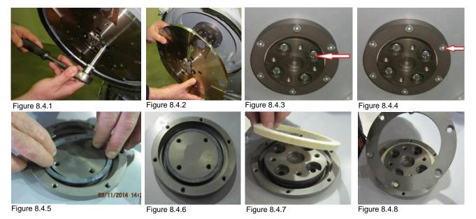
To check or replace the buffers and the elastic elements, the tool holders have to be dismounted.
